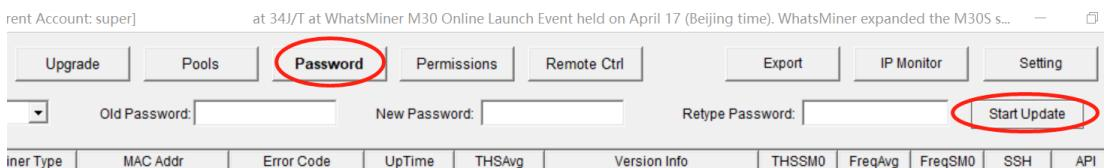
The screenshot shows the main interface of WhatMinerTool. At the top, there are several tabs: Upgrade, Pools, Password, Permissions, Remote Ctrl, Export, IP Monitor, and Setting. The 'Password' tab is highlighted with a red circle. Below the tabs, there are input fields for Old Password, New Password, and Retype Password, followed by a 'Start Update' button, which is also circled in red.
